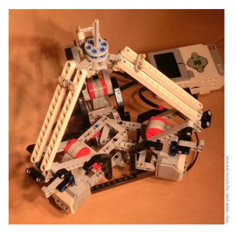
Positioning accuracy is disappointing (at least by delta robot standards), even though care has been taken to make the chassis very rigid with three layers of beams and rectangular frames interlocking at 120°. Still, this model is a good introduction to parallel robot kinematics. For better accuracy, gear reduction and pre-tensioning should be considered.
