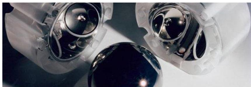
Gravity Probe B gyroscope rotor
