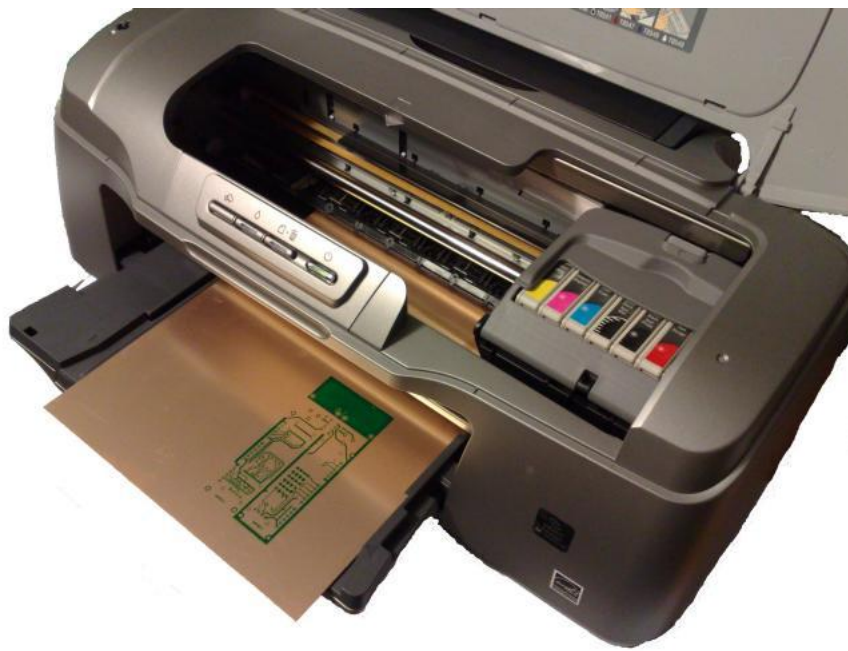
Figure 1. Unmodified Epson R800 printing on 200x300 mm copper-clad epoxy.
