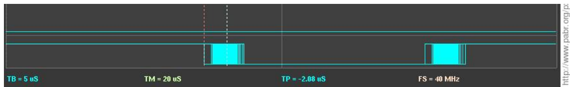
Figure 5. 20 \mu s pulses generated by pxa_rtsched, with \pm 2 \mu s jitter
