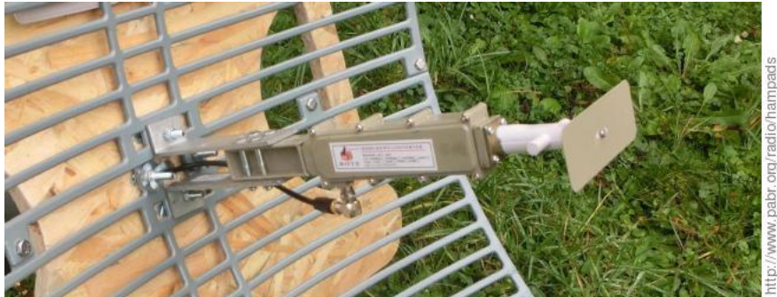
Figure 3. MMDS LNB attached to grid-parabolic Wi-Fi reflector
