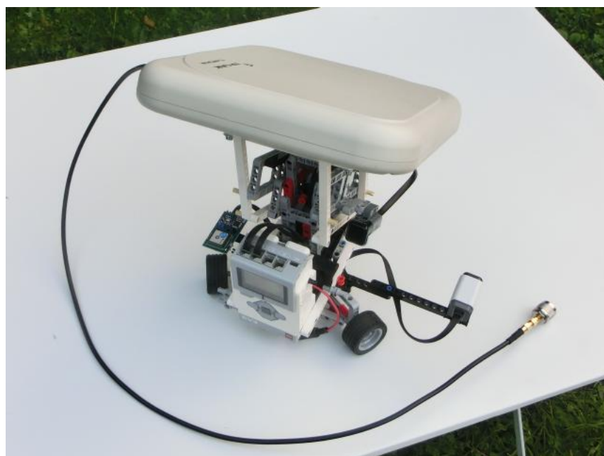
Figure 8. LEGO tracker for LEO satellites
