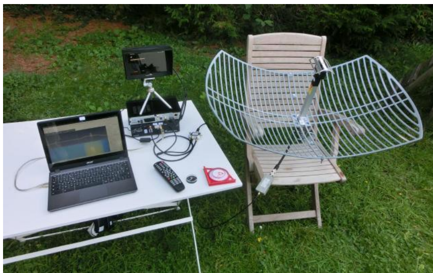
Figure 1. Setup with fixed 24 dB antenna
