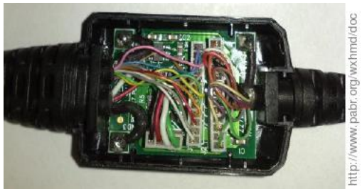
Figure 4. Circuit board hidden inside the cable
